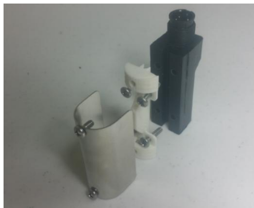
Figure – 5: CS-HE-150 assembly with Module, Stabilizer and Shield
