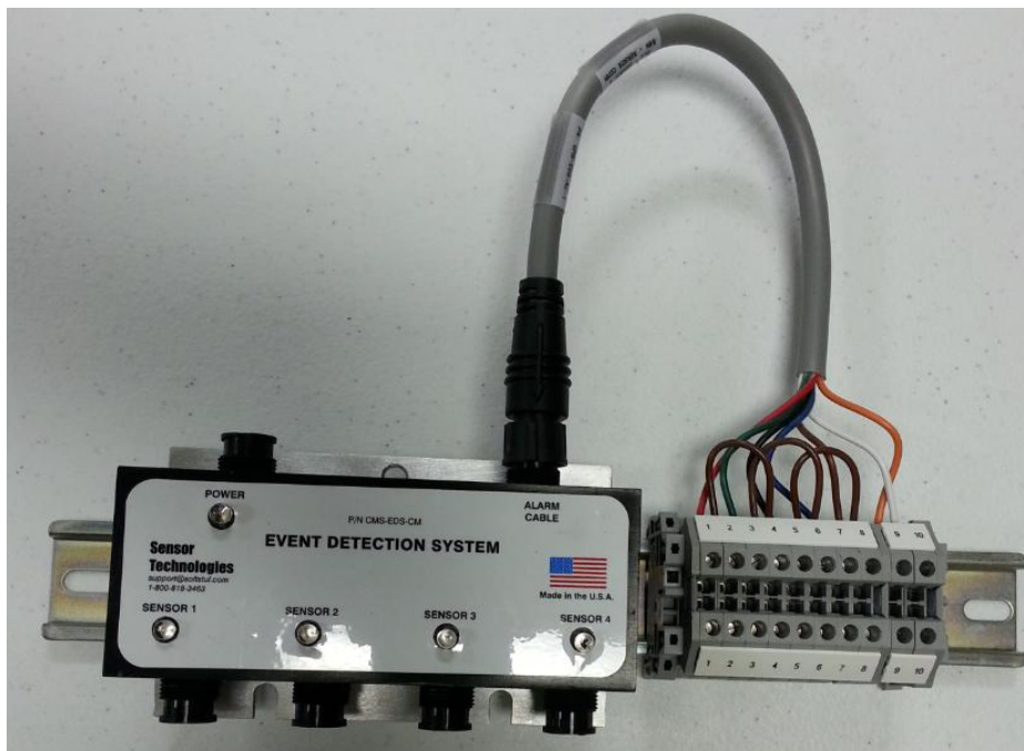
Figure 3: Control Module with Terminal Block and Alarm Cable
